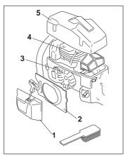
Clean the cooling system with a brush once a week, more often in demanding conditions. A dirty or blocked cooling system results in the saw overheating which causes damage to piston and cylinder.
